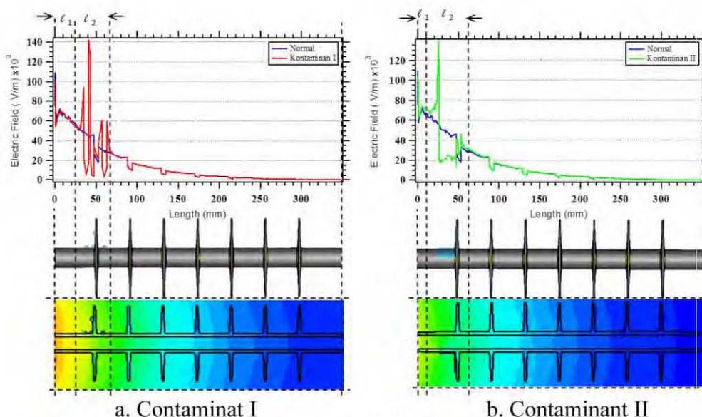
Figure 1. Electric field distribution on the surface of insulator
